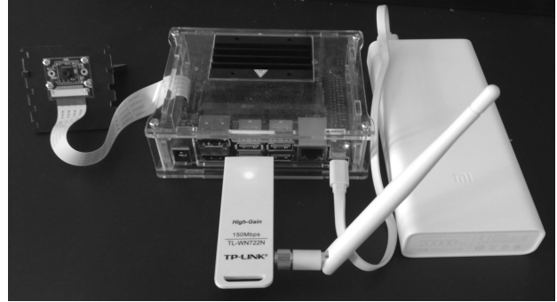
Fig. 2. IoT monitoring device used for bee observation and varroosis detection.
