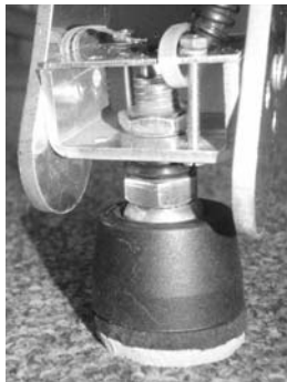
Fig. 19. Example application of the pressure sensor on the Messor robot.
