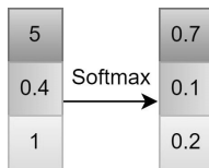
Fig. 5. Illustration of the softmax operation.
