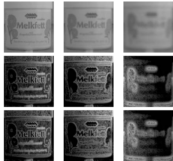
Fig. 6. Example of a scene with a bright object and reduced perceived contrast. Top row: object in focus and moving away, middle row: gradient image obtained with the LTIP Laplacian, bottom row: gradient image obtained with the Vollath F4 function. Typically, our method produces a more accurate but flatter FMF, while Vollath—sharper but with fake modes.
