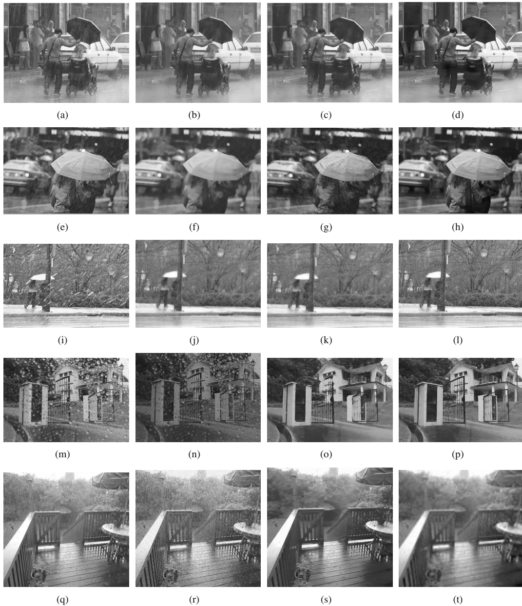
Fig. 5. Deraining results of various deraining networks on five synthetic data sets.
